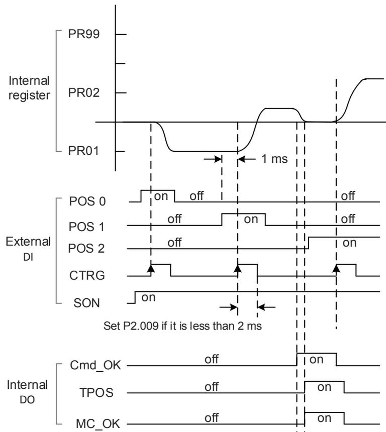
Note: Cmd\_OK is on when the PR command completes; TPOS is on when the error is smaller than value set by P1.054; MC\_OK is on when Cmd\_OK and TPOS are both on.
