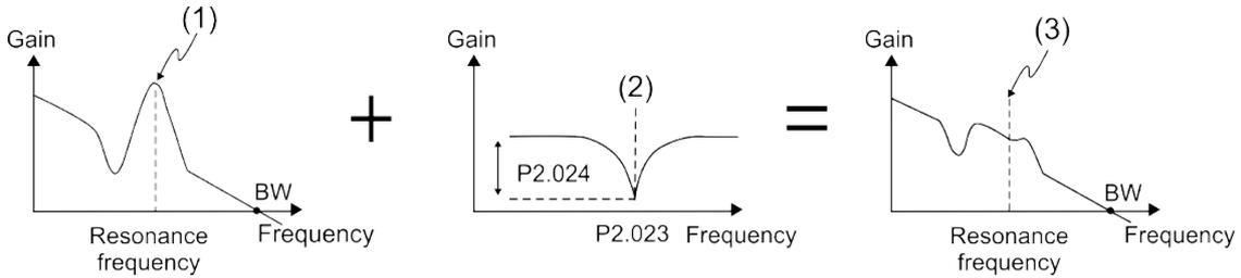
(1) Point of resonance (2) Notch filter (3) Point of resonance suppressed by the Notch filter
