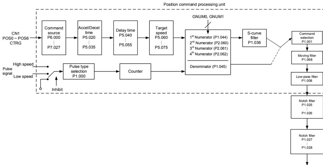
The upper path of the above diagram is the PR mode and the lower one is the PT mode that you can select with P1.001. You can set E-Gear ratio in both modes to adjust the positioning resolution. In addition, you can use either an S-curve or low-pass filter to smooth the command (described below).
