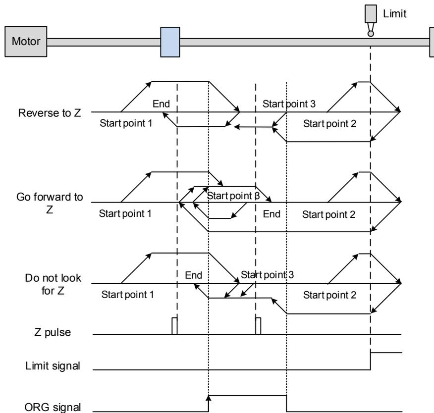
The figure above shows an example of reversing to look for the Z pulse. If the home sensor signal for the start position is un-triggered (low, Start point 1), the servo motor operates at high speed (first speed setting) until it reaches the rising-edge of ORG signal. Then it decelerates, switching to low speed (second speed setting) and reverses to look for the Z pulse. When the motor finds the Z pulse, it decelerates to a stop, completing the homing.
