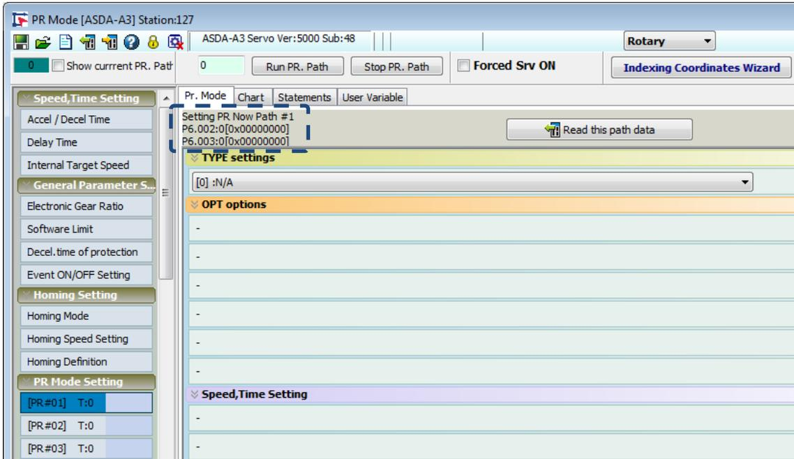
Figure 7.1.2 PR mode interface in ASDA-Soft
