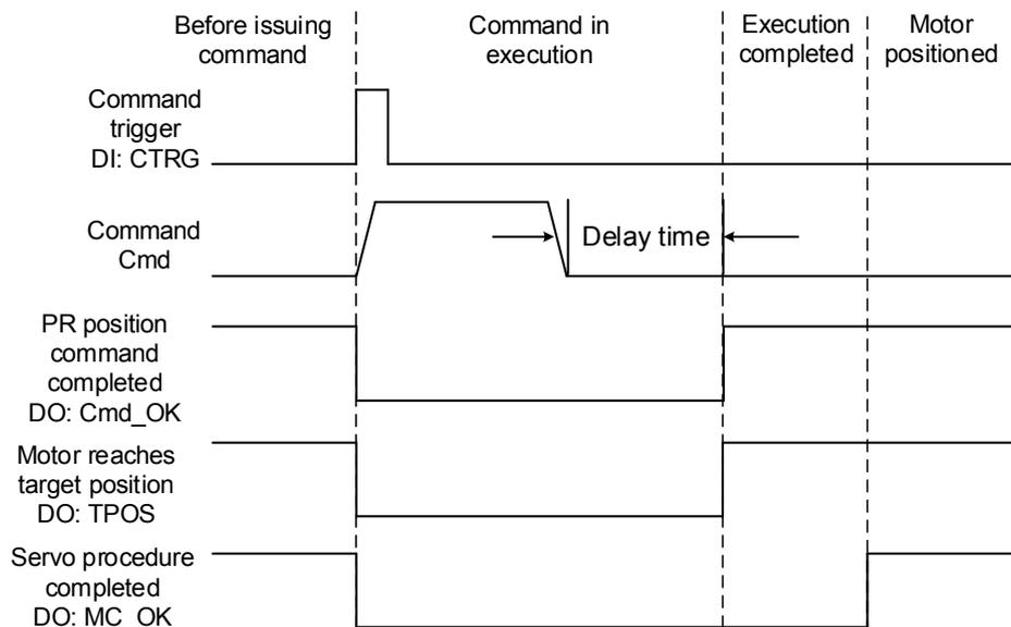
Figure 7.1.2.3 Operation of DI/DO signals in PR mode
