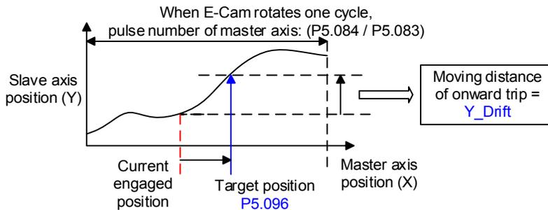
Note: regardless of onward trip or return trip, use the PR command through incremental positioning control. Due to cyclic operation, when E-Cam moves from current position to the target position, it can either rotate in the forward or reverse direction. However, the moving distance is usually different between them. Thus, you can use the allowable forward rate to determine whether to operate in forward or reverse rotation.
