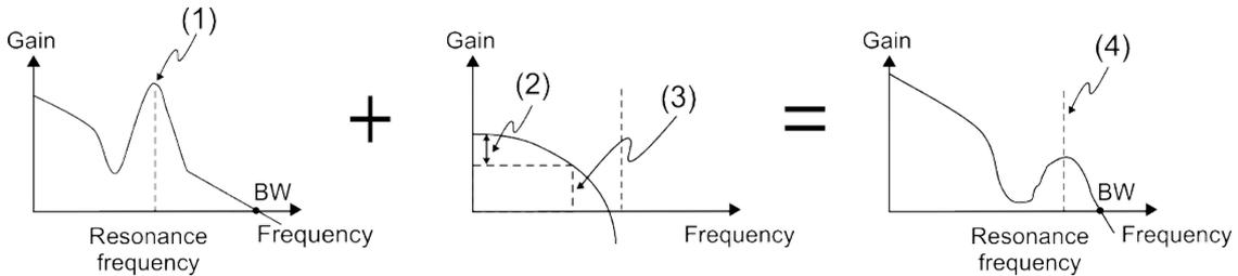
(1) Point of resonance (2) Attenuation rate (-3 dB)
