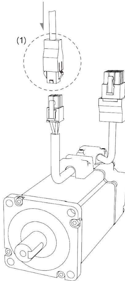
Note: pin assignments of the A3 and A2 model are the same. For easier wiring, A3's connector illustration (angle of viewing) is changed, which is different from that of A2.
