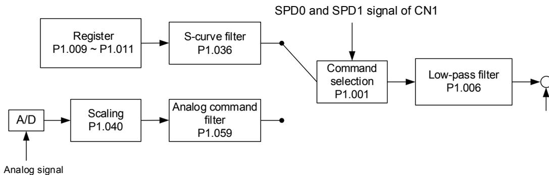
Control in the upper path is from the register while the in lower path it is from the external analog voltage. The command is selected according to the status of SPD0, SPD1 and P1.001 (S or Sz). In this condition, the S-curve and low-pass filters are applied to achieve a smoother response.
