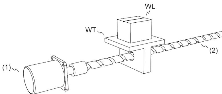
(1) Motor (2) Ball screw pitch: 3 mm (equals 3000 μm)
