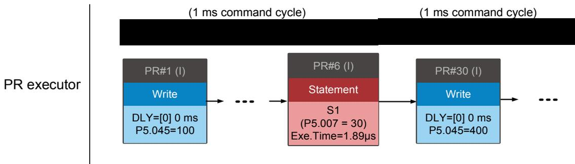
Figure 7.1.6.13 Writing trigger command in Statement section
