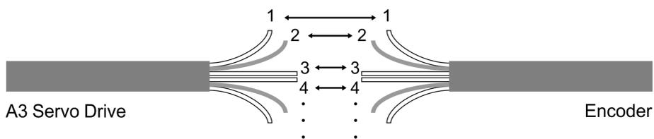
To directly connect the wires without using the connectors, please wire them according to the corresponding wire number (shown above). For example, connect wire No. 1 of the servo drive to No. 1 of the motor encoder; connect wire No. 2 of the servo drive to wire No. 2 of the motor encoder and so on. Please number the wires of the servo drive in sequence and then connect them to the encoder.
