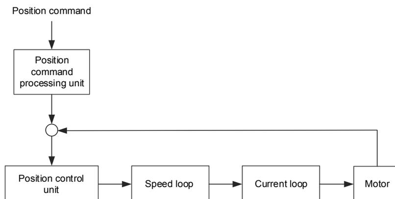
For better control, the pulse signals are processed by the Position Command processing unit. The structure is shown in the diagram below.
