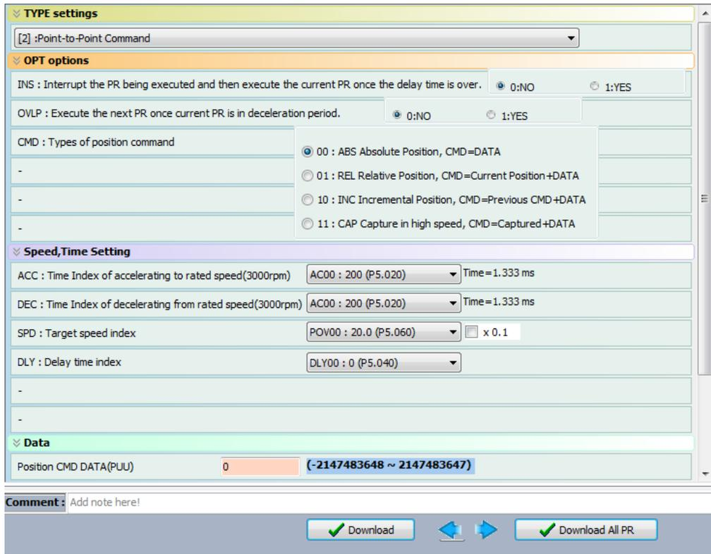
Figure 7.1.3.6 PR mode position interface of ASDA-Soft
