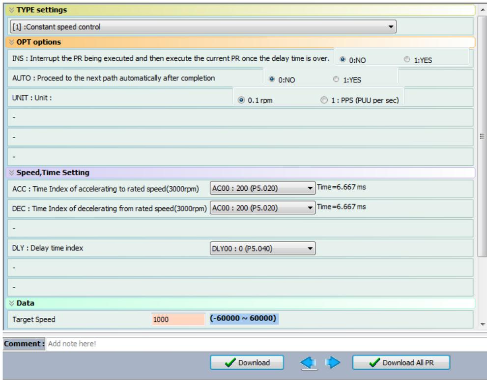
Figure 7.1.3.4 PR mode Speed screen in ASDA-Soft
