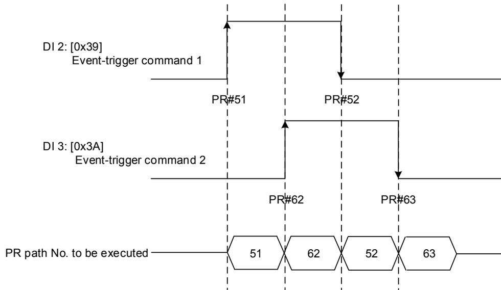
Figure 7.1.5.3 Example of Event triggering timing diagram
