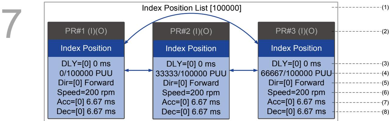
Figure 7.1.4.7 Indexing Position command display
