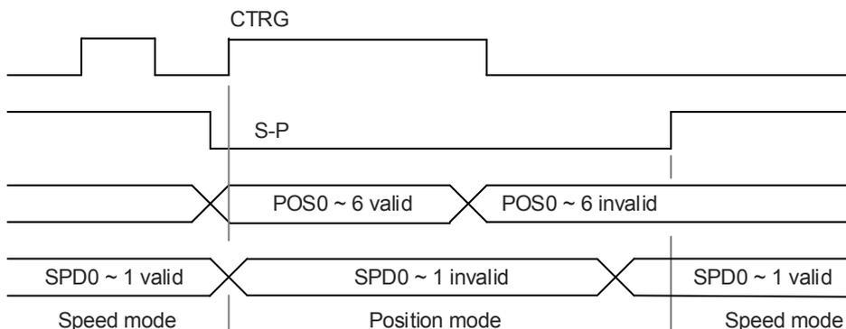
Figure 6.5.1.1 Speed / Position dual mode
