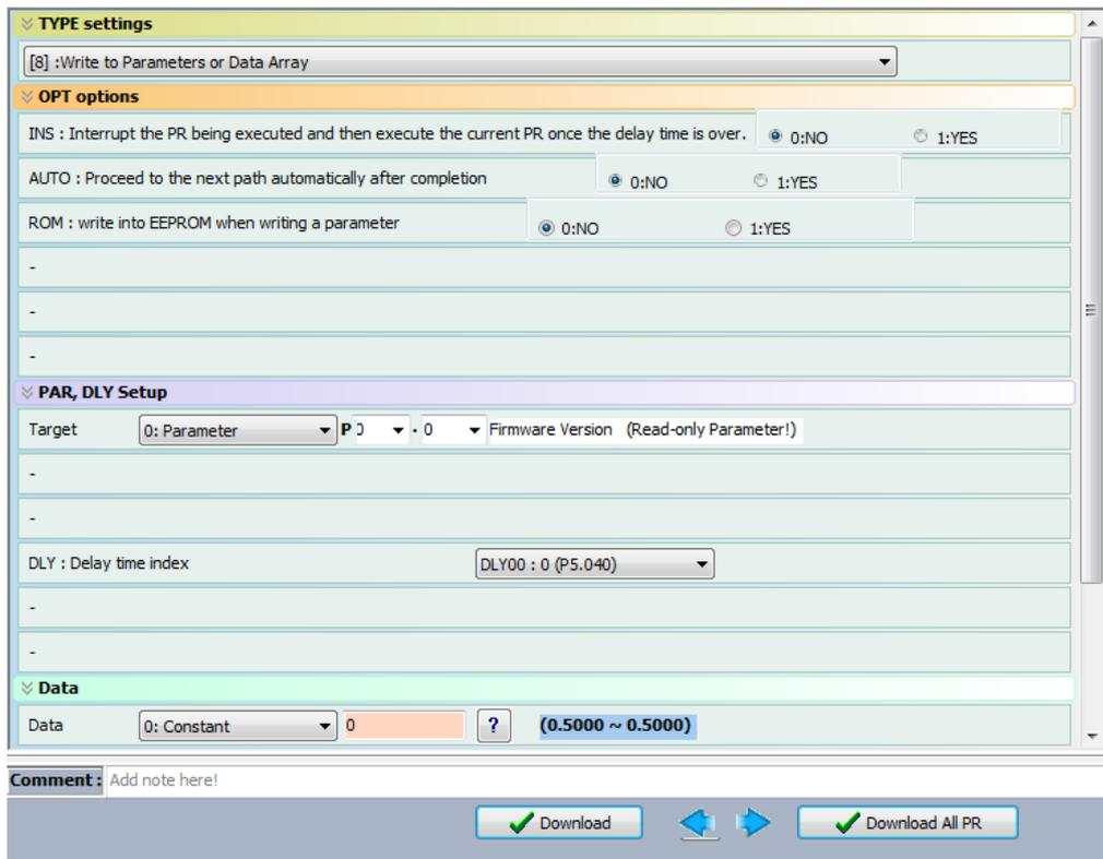
Figure 7.1.3.11 Using PR Write command in ASDA-Soft
