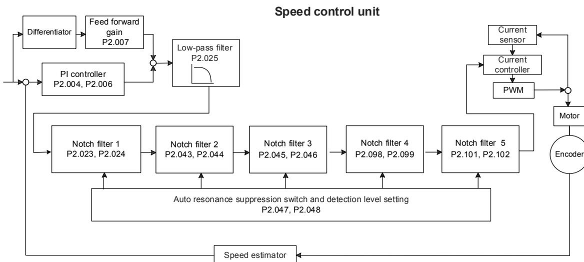
The ASDA-A3 provides two types of resonance suppression: one is the Notch filter and the other is the low-pass filter. See the following diagrams for the results of using these filters.
