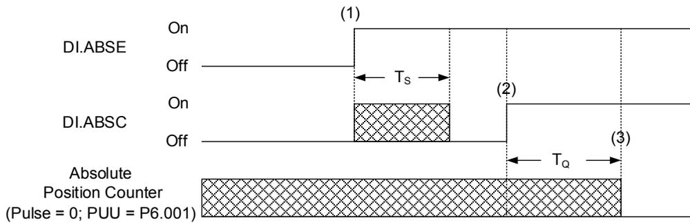
Figure 10.3.4.1 Timing diagram for initializing the absolute coordinate system with DI/DO
