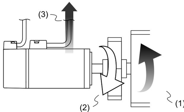
(1) Direction of motion of the object; (2) Force direction of the motor; (3) Regenerative power
