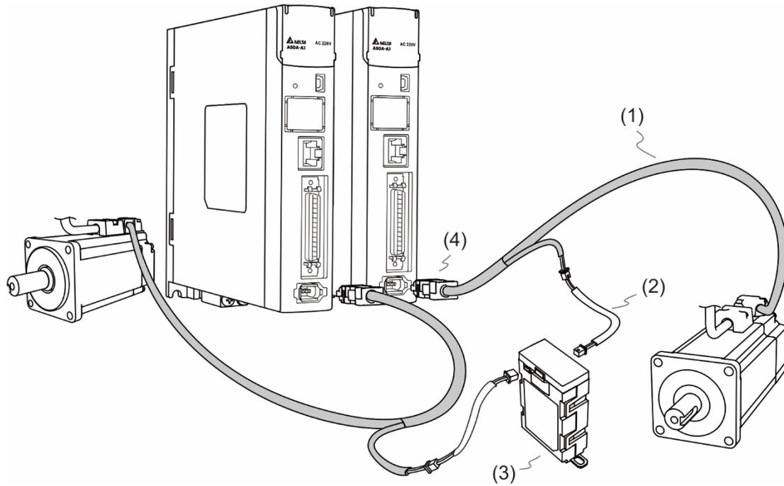
(1) Encoder cable; (2) Battery box cable AW; (3) Double battery box (absolute type); (4) CN2 connector
