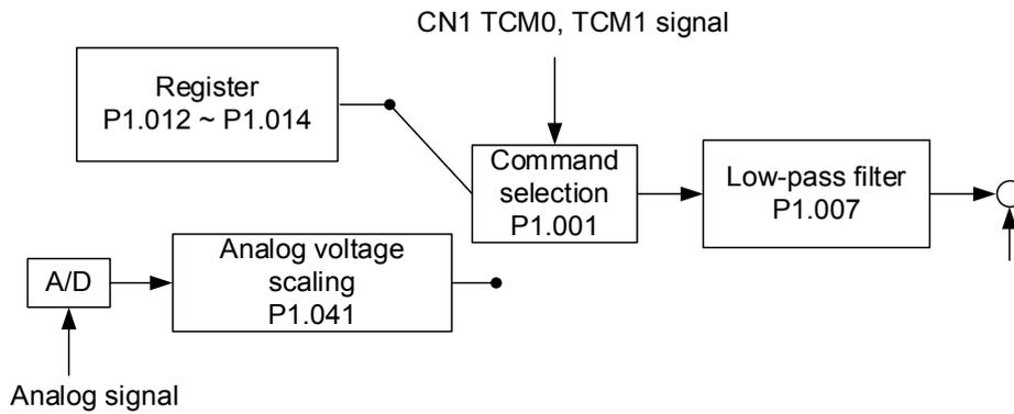
Control in the upper path is from the register while the in lower path it is from the external analog voltage. You select the command according to the status of TCM0, TCM1, and P1.001 (T or Tz). You can adjust the torque with the analog voltage scaling (P1.041) and you can smooth the response with the low-pass filter (P1.007).
