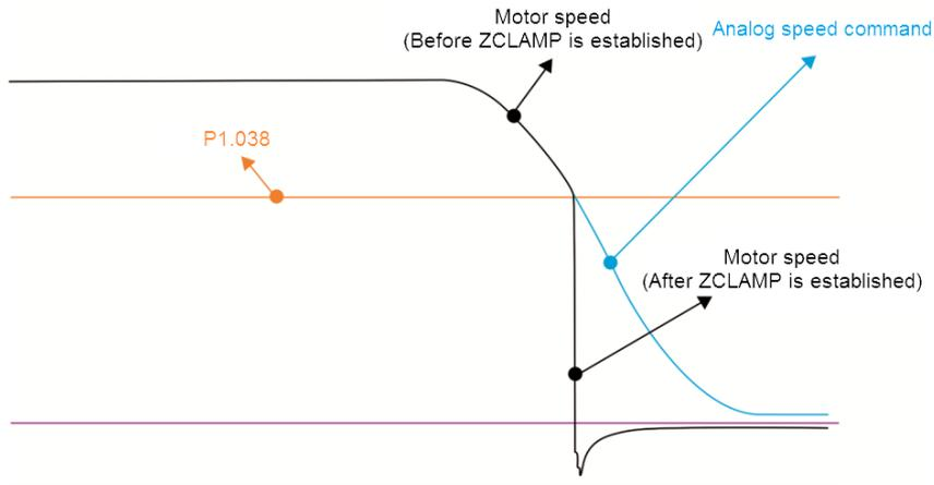
1: command source is the analog voltage. ZCLAMP function uses the analog Speed command without acceleration / deceleration to determine if this function is enabled. When ZCLAMP conditions are met, the motor speed decelerates to 0 rpm by S-curve deceleration. If ZCLAMP conditions are not met, the motor follows the analog Speed command through the S-curve.
