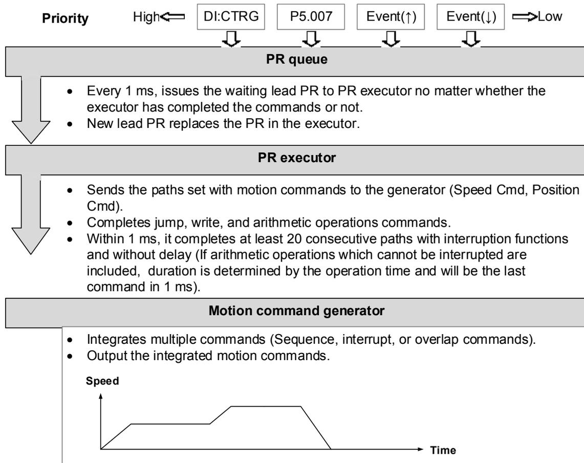
Figure 7.1.6.1 PR execution flow in the ASDA-A3
