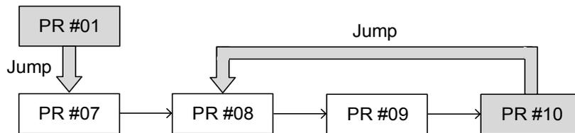
Figure 7.1.3.9 Jump command in PR mode
