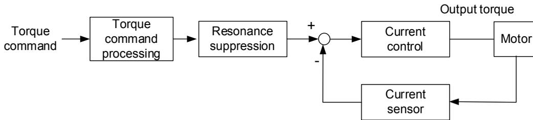
You use the Torque Command unit to specify the Torque command source (mentioned in Section 6.4.1), including the scaling of the analog voltage (P1.041) and the S-curve setting. The current control unit manages the gain parameters for the servo drive and calculates the current for servo motor in real-time; you can only set this by commands.
