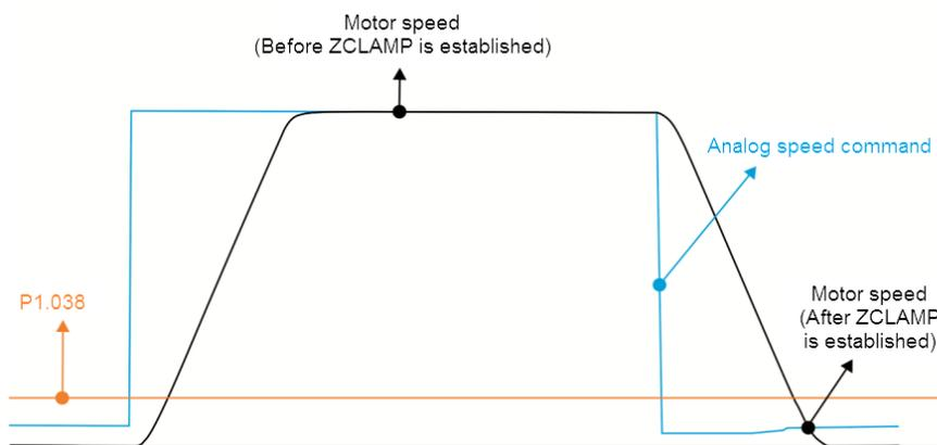
1: command source is the internal register. ZCLAMP function uses the register Speed command with acceleration / deceleration to determine if this function should be enabled. When ZCLAMP conditions are met, the motor speed is set to 0 rpm.
