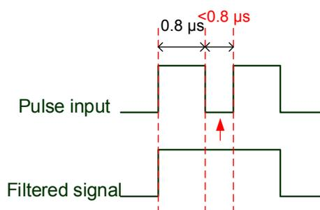
If this low level pulse width is shorter than 0.8  $\mu$ s, it may be filtered, and thus two input pulses will be regarded as one pulse. If this low level pulse width is shorter than 0.2  $\mu$ s, it will be filtered.
