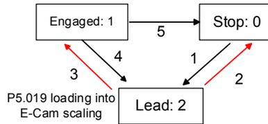
If necessary in the application, there are two ways to change the setting of E-Cam curve scaling immediately:
