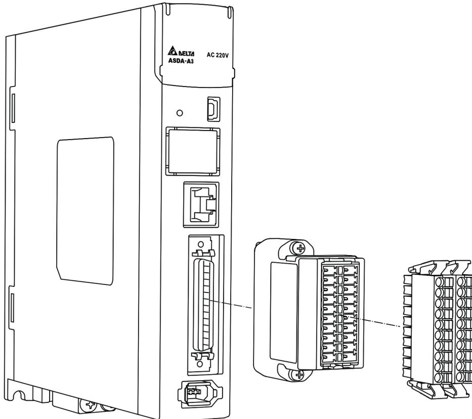
Pin assignment for the CN1 quick connector (J2 and J1):
