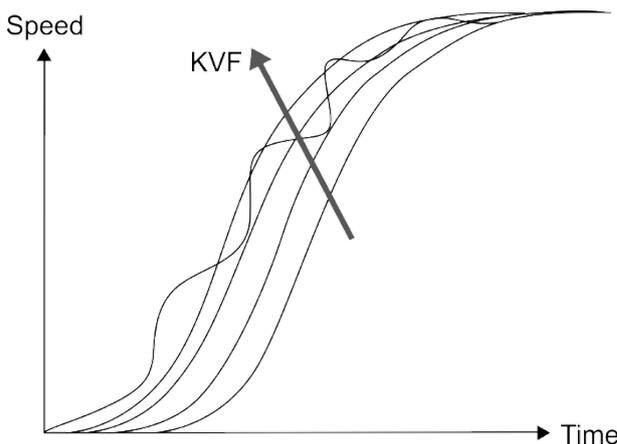
The closer the KVF value is to 1, the more complete the forward compensation. The following error becomes very small. But a KVF value that is set too high also causes vibration.
