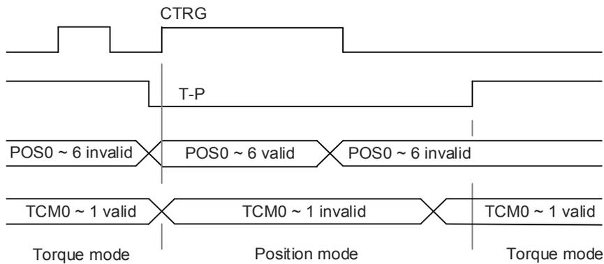
Figure 6.5.3.1 Torque / Position dual mode
