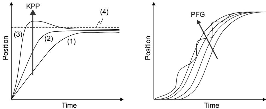
The actual position curve changes from (1) to (3) with the increase in the KPP value. (4) stands for the Position command.
