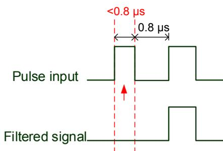
If this first pulse width is shorter than 0.8  $\mu$ s, it may be filtered, and thus two input pulses will be regarded as one pulse. If this pulse width is shorter than 0.2  $\mu$ s, it will be filtered.
