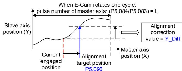
\*P5.093.UZ is able to limit the maximum correction rate. The alignment target position ★ will be different from P5.096.
