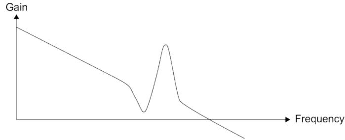
When the value of P2.025 is increased from 0, BW becomes smaller. Although it solves the problem of the resonance frequency, the response bandwidth and phase margin are reduced. Also, the system becomes unstable.
