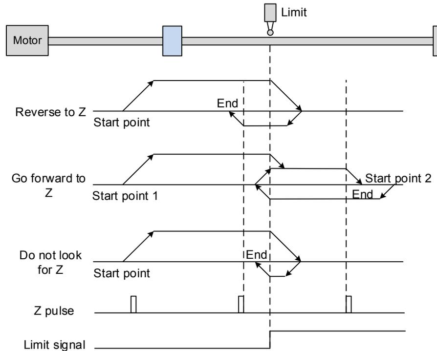
In the example above (looking for the Z pulse), the servo motor operates at high speed (first speed value) and then decelerates once it reaches the limit (rising-edge triggers the signal). Then the motor switches to low speed (second speed value) to look for the Z pulse. When the motor finds the Z pulse, it decelerates and stops, completing the homing procedure.
