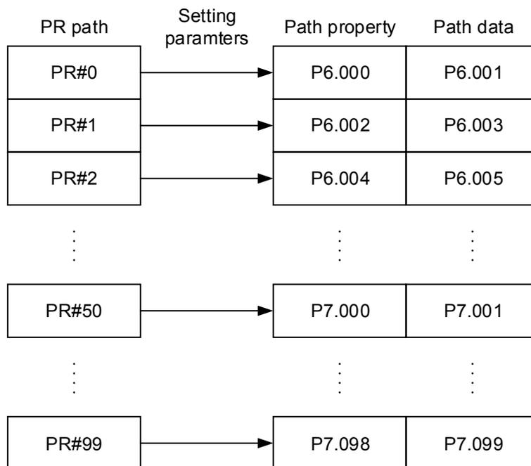
Figure 7.1.1 Setting parameters for each PR path
