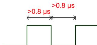
When the high or low duty width of the pulse is smaller than the filter width, then it is filtered out.
