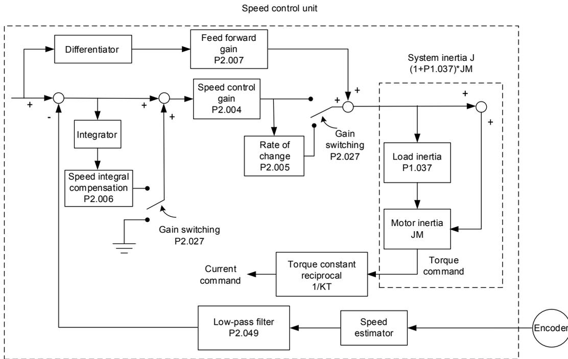
In the Speed Control unit, you can adjust different types of gain. You can adjust the gain manually or use the three gain adjustment modes provided.
