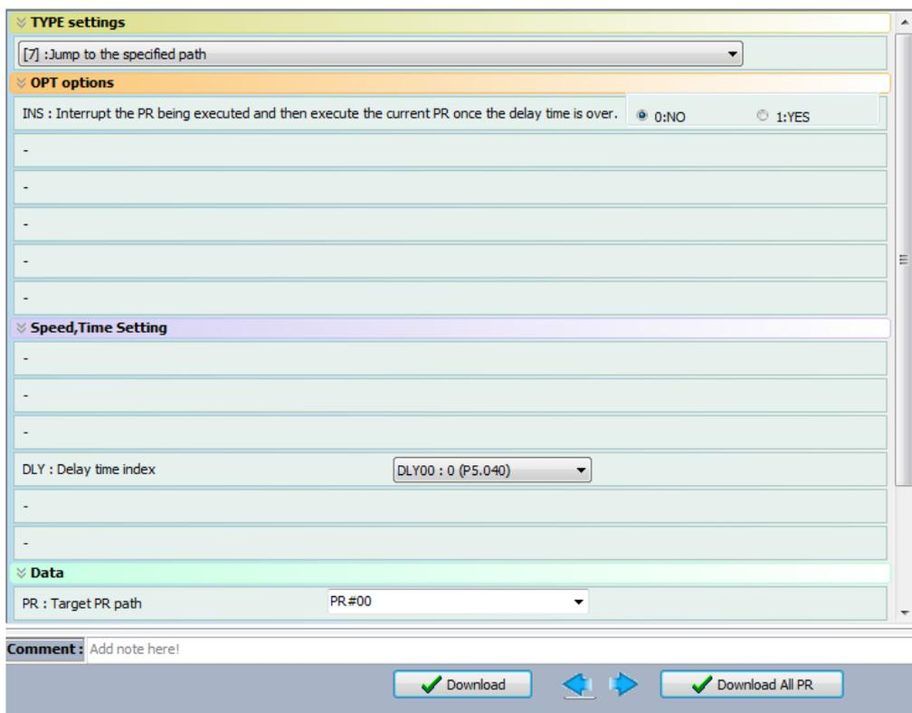
Figure 7.1.3.10 Using PR mode Jump command in ASDA-Soft
