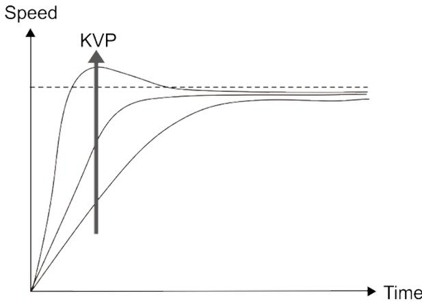
The higher the KVP value, the larger the bandwidth. The time of the speed increase will also be shorter. However, if the value is set too high, the phase margin is too small. The effect is not as good as KVI for the steady-state error but is better for the effect on following.
