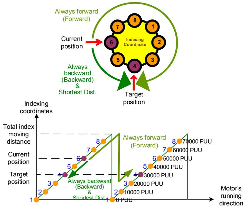
Figure 7.1.3.15 Motor's operation direction and indexing coordinates
