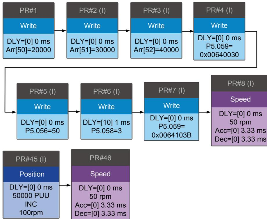
Figure 7.2.3.3 PR path using the Compare function
