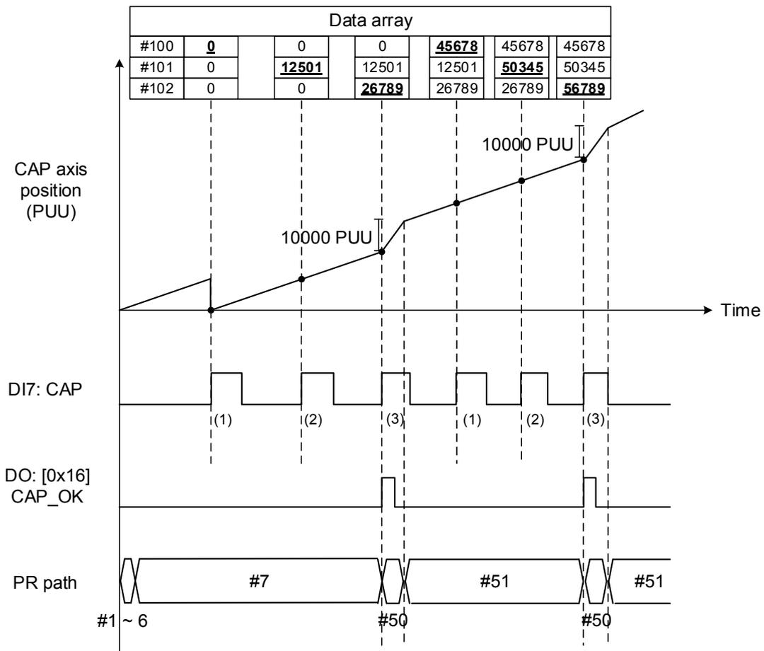
Figure 7.2.2.4 Application example for high-speed capturing function
