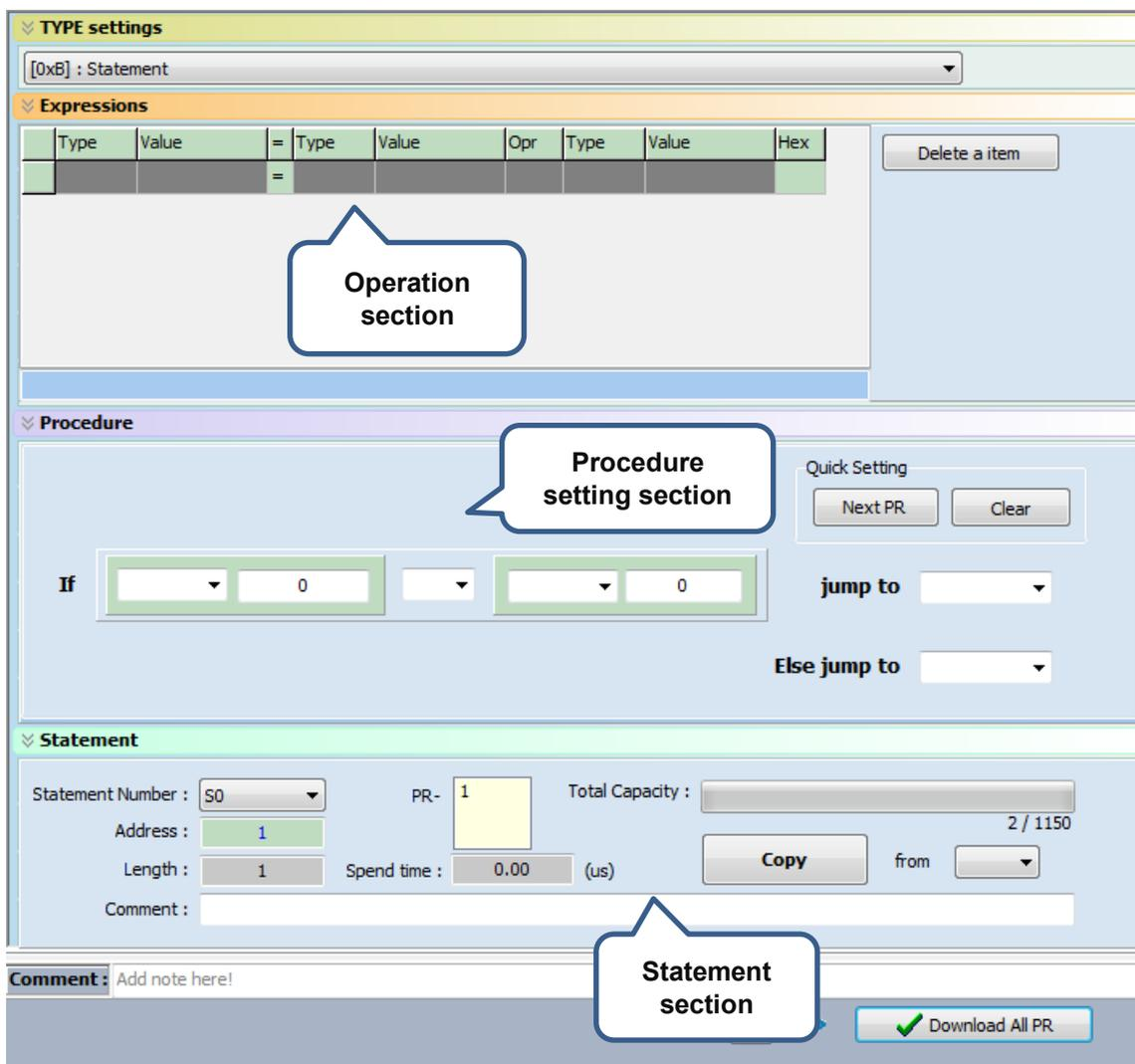
Figure 7.1.3.16 PR Arithmetic Operations screen in ASDA-Soft
