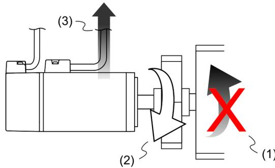
(1) Direction of motion of the object; (2) Force direction of the motor;
