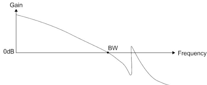
If you know the resonance frequency, the Notch filter can eliminate the resonance directly. The frequency range of the notch filter is 50 – 5000 Hz and the suppression strength is 0 – 32 dB. If the frequency does not meet the Notch filter conditions, then using the low-pass filter to reduce the resonance is suggested.
