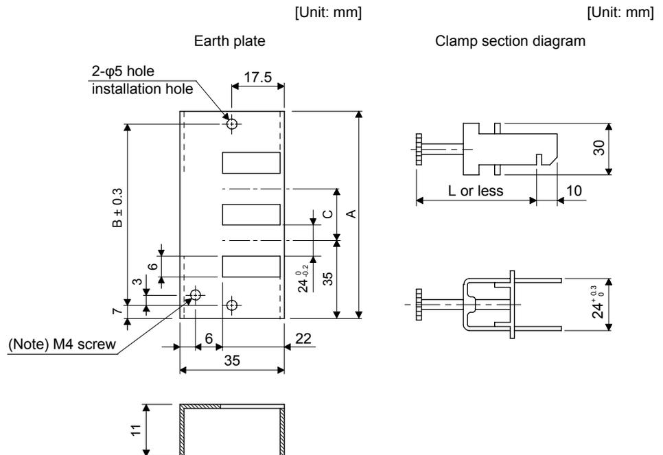
Note. Screw hole for grounding. Connect it to the grounding plate of the cabinet.
