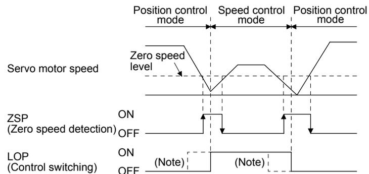
Note. When ZSP is not turned on, the control mode is not switched even if LOP is turned on/off. After LOP is turned on/off, even if ZSP is turned on, the control mode is not switched.
