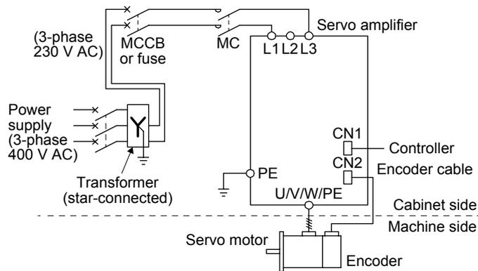
The control circuit connectors described by rectangles are safely separated from the main circuits described by circles.
