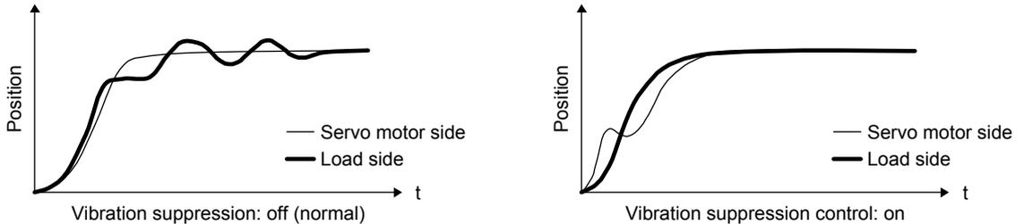
When the advanced vibration suppression control II ([Pr. PB02 Vibration suppression control tuning mode]) is executed, the vibration frequency at load side is automatically estimated to suppress machine side vibration two times at most.
