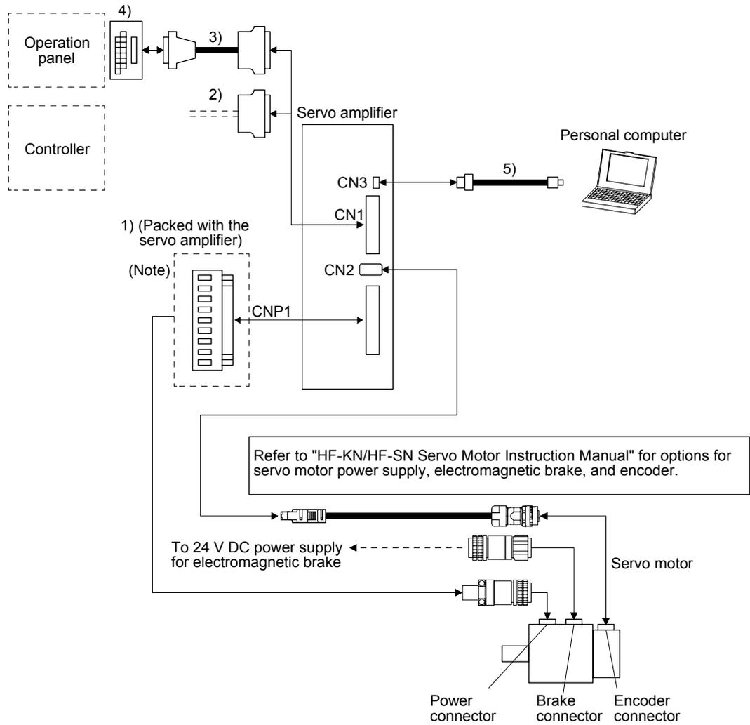
Note. Connectors for 1 kW or less. Refer to section 3.3.3 (1) (b) for 2 kW or more.
