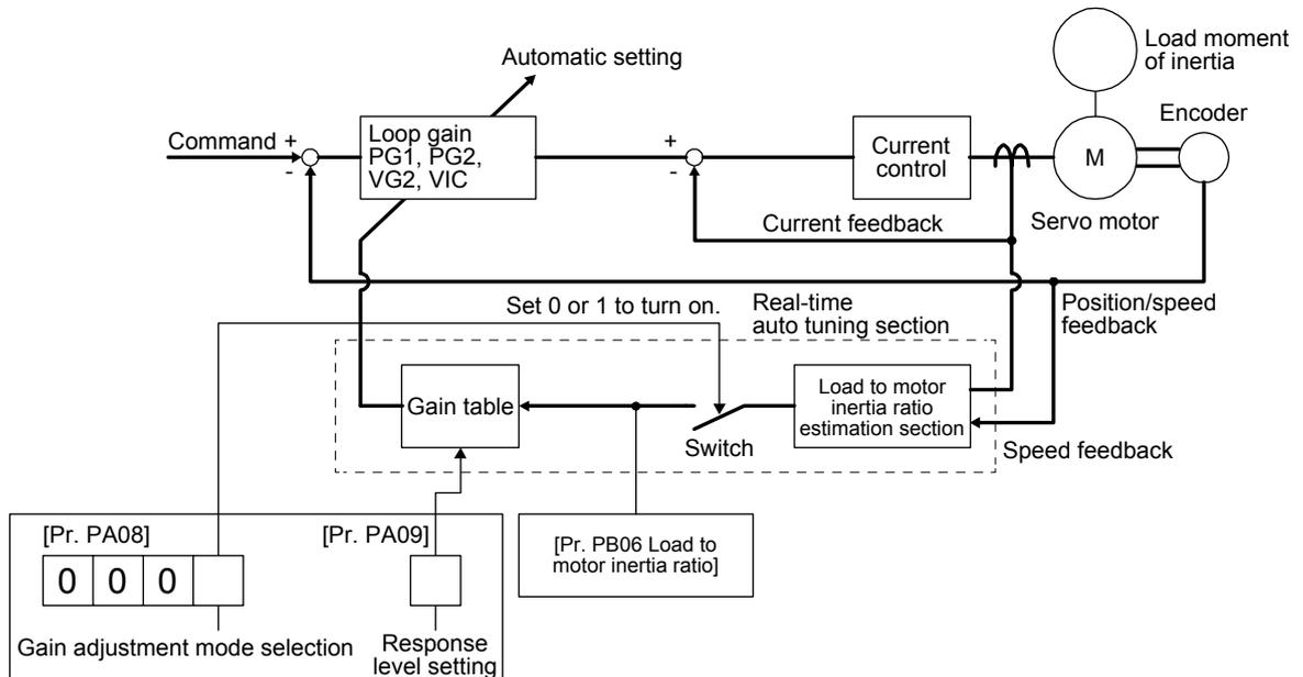
When a servo motor is accelerated/decelerated, the load to motor inertia ratio estimation section always estimates the load to motor inertia ratio from the current and speed of the servo motor. The results of estimation are written to [Pr. PB06 Load to motor inertia ratio]. These results can be confirmed on the status display screen of the MR Configurator2.
