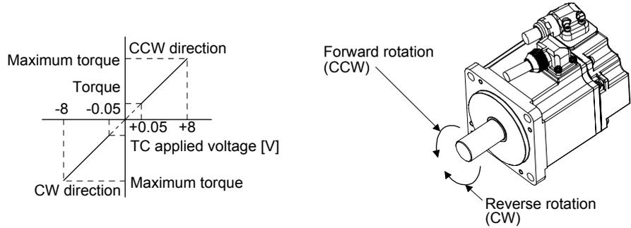
Generated torque command values will vary about 5% relative to the voltage depending on products. The torque may vary if the voltage is low (-0.05 V to 0.05 V) and the actual speed is close to the limit value. In such a case, increase the speed limit value.
