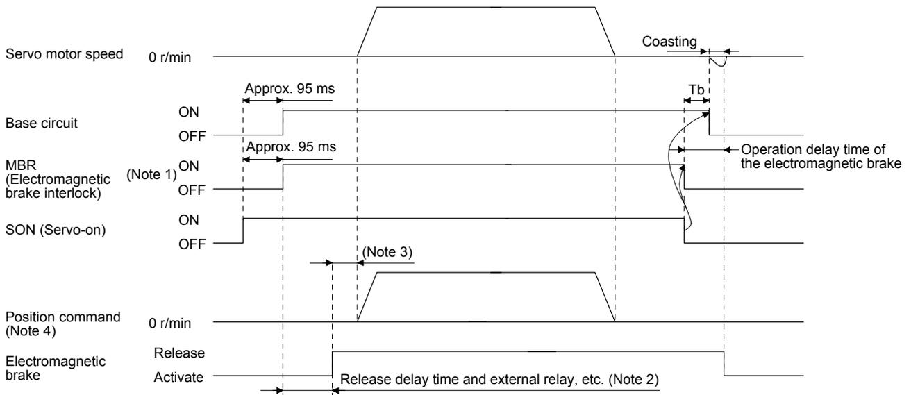
Note 1. ON: Electromagnetic brake is not activated.
