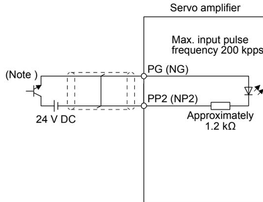
Note. Pulse train input interface is comprised of a photocopler.
