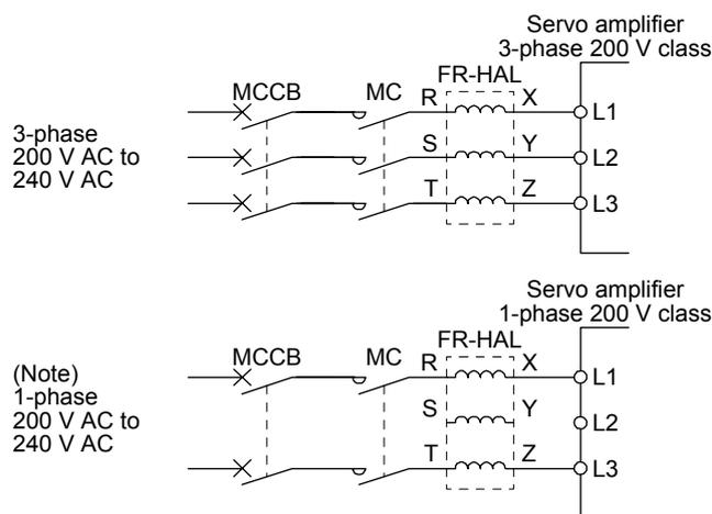
Note. For 1-phase 200 V AC to 240 V AC, connect the power supply to L1 and L3. Leave L2 open.
