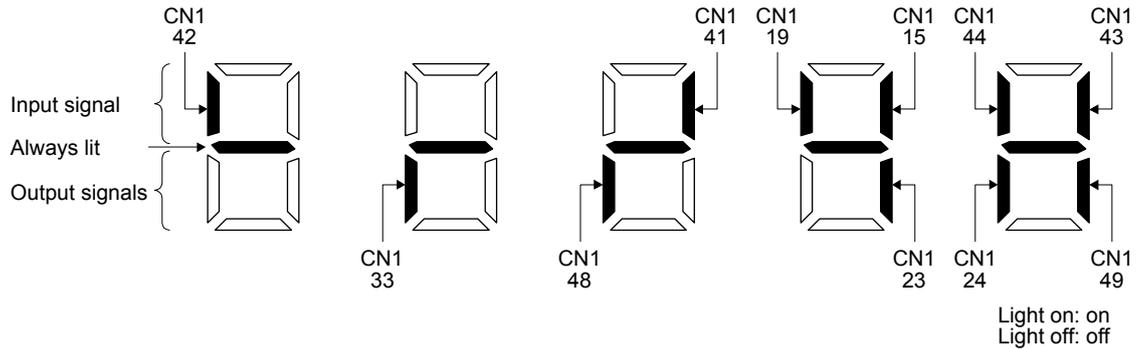
The LED segment corresponding to the pin is lit to indicate on, and is extinguished to indicate off. The signals corresponding to the pins in the respective control modes are indicated below.
