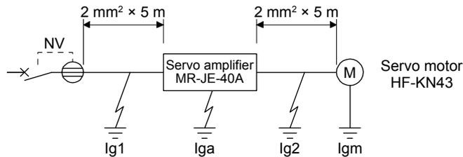
Use an earth-leakage current breaker designed for suppressing harmonics/surges. Find the terms of equation (11.1) from the diagram.
