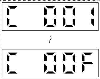
If an error occurs during the one-touch tuning, the tuning will be forcibly terminated and the stop symbol and error code from "C 001" to "C 00F" will be displayed by turns with 2 s interval.
