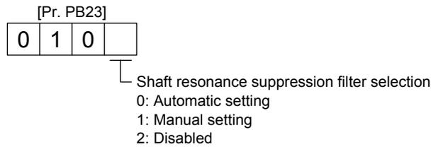
To set [Pr. PB17 Shaft resonance suppression filter] automatically, select "Automatic setting".
