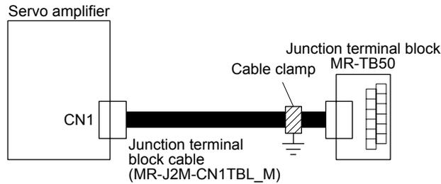
Install the junction terminal block cable on the junction terminal block side with the supplied cable clamp fitting (AERSBAN-ESET). For the use of the cable clamp fitting, refer to section 11.9, (2) (c).
