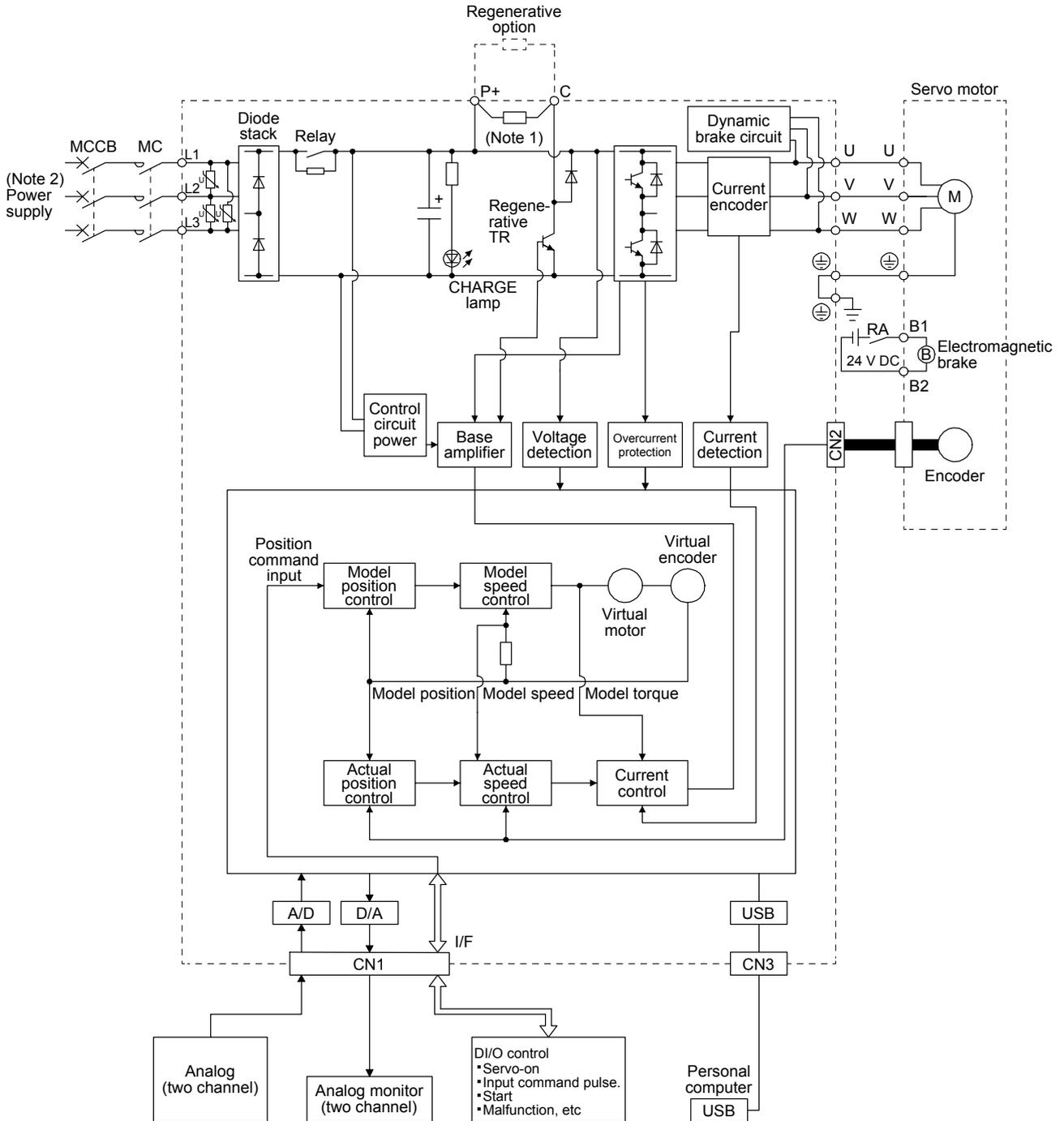
Note 1. The built-in regenerative resistor is not provided for MR-JE-10A and MR-JE-20A.
