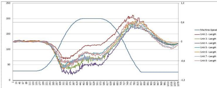
Register Error – 8 PU Machine – Material PE
