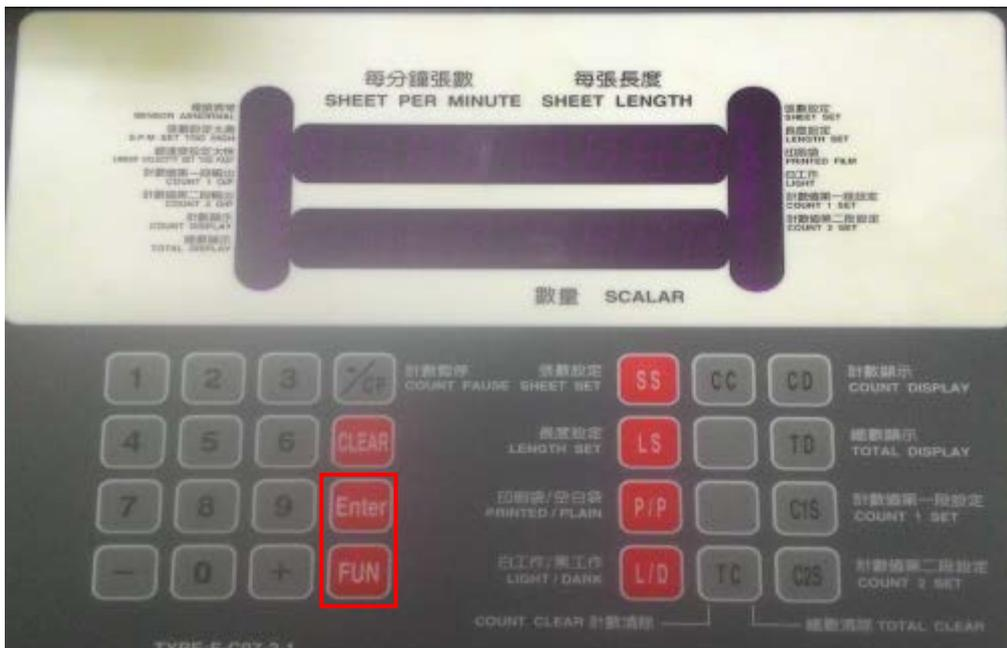
Step 2: The parameter adjustment of controller C07-2C and C07-5
