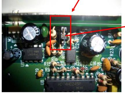
此處可調整音量大小 例:原 1&2 腳有插 JAMP,請將 JAMP 拔起 插至 2&3 腳 Adjust the volume form here. Please take off the original JAMP in pin 1 and 2. Then JAMP plugs in pin 2 and 3.
